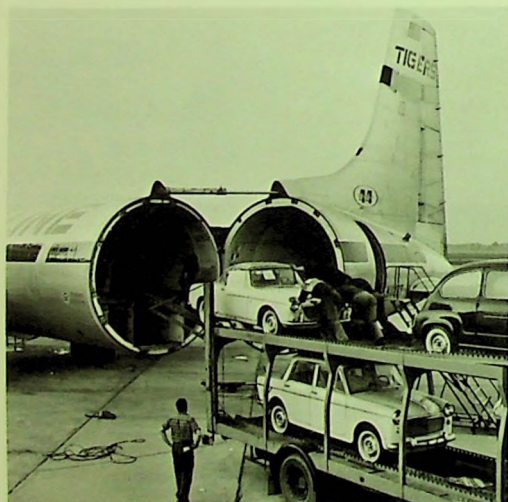
Part of a planeload of compact cars is rolled directly from truck carry-all into CL-44 cargo hold.
