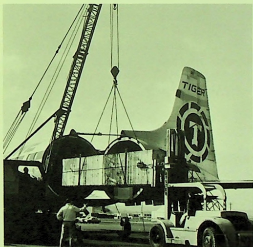
Big size freight like this part of a Polaris missile is made to order for Flying Tiger's CL-44, the only commercial aircraft which can handle such shipments.
