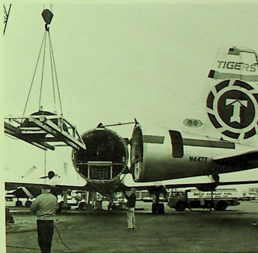
Rigging crane is used to load part of a 57,000-pound General Electric turbine shipment, largest ever flown, for the Southern California Edison Co., aboard CL-44 at Newark. No other type of airfreighter could have handled such a shipment.
