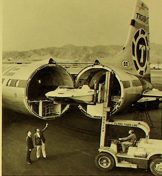
Burbank, Calif.—New-type racing hydroplane being loaded aboard CL-44D. Note how air shipment permits uncrated handling of boat, thus greatly reducing shipping costs.
