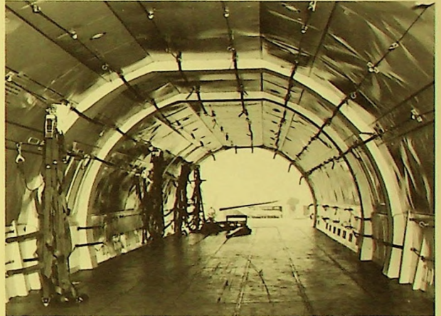
Interior view of CL-44D main cargo hold, which is 98 feet long, including swingtail compartment, 11½ feet wide and 6¾ feet high. Rigging on left is cargo netting used to secure freight.
