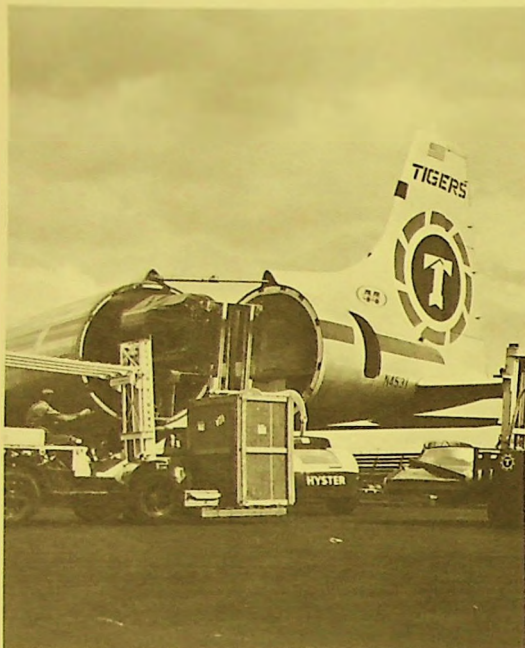
Big freight, as well as small, goes easily through the swingtail of a Flying Tiger CL-44D prop-jet, mainstay of the Tiger freight fleet.
