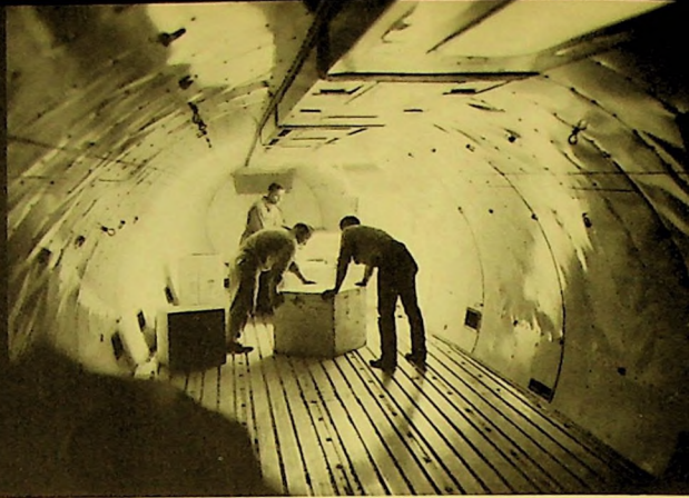
A portion of the interior of a Constellation airfreighter. The total cubic capacity is equal to two 40-ft. box cars.
