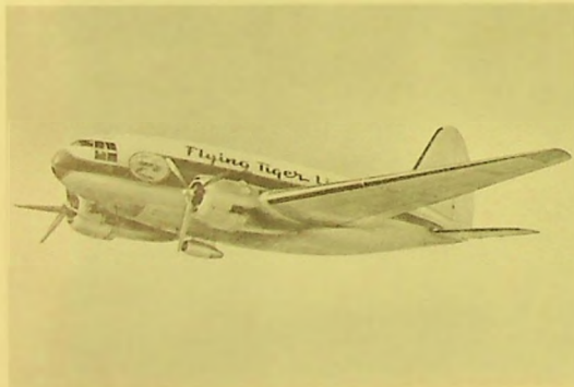
The experimental C-46 aloft, propellers feathered, powered only by the turbojet.
