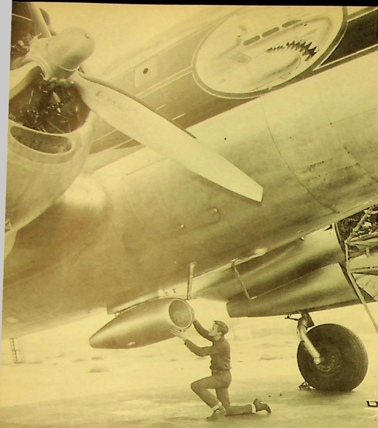
The experimental turbojet, designed to provide more power and greater safety for a C-46.
