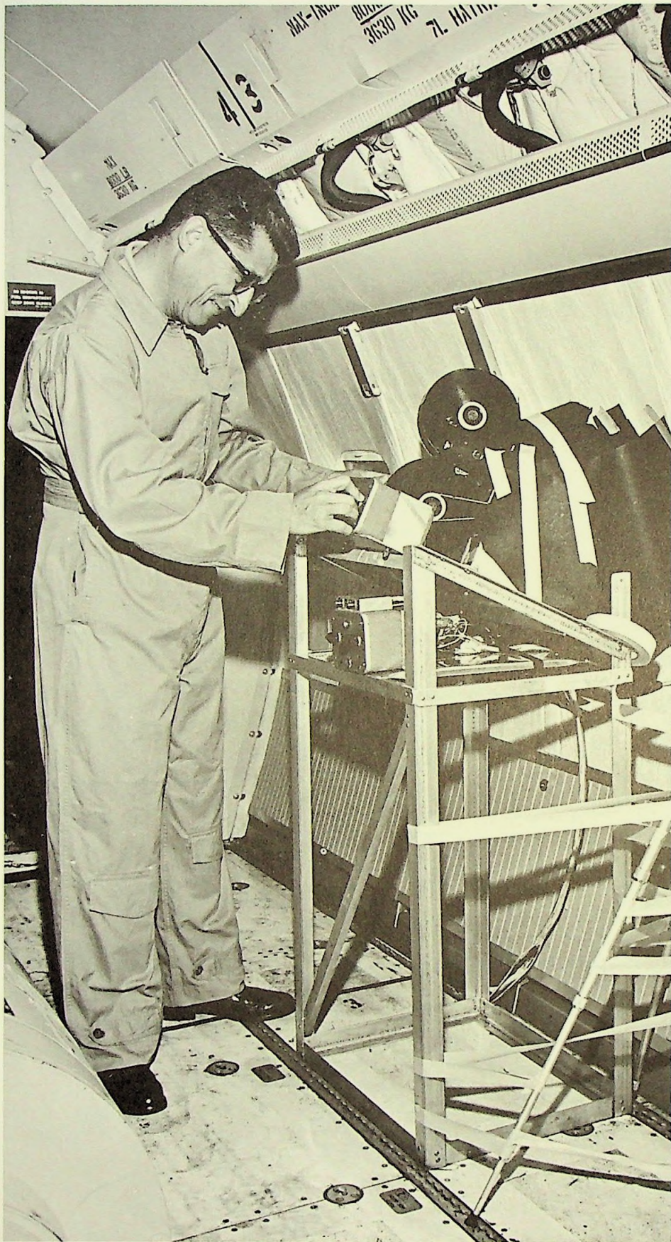
Peter Mesquita, scientist for Litton Industries, makes final check of time lapse cameras and other photographic equipment used on the Boeing 707.
