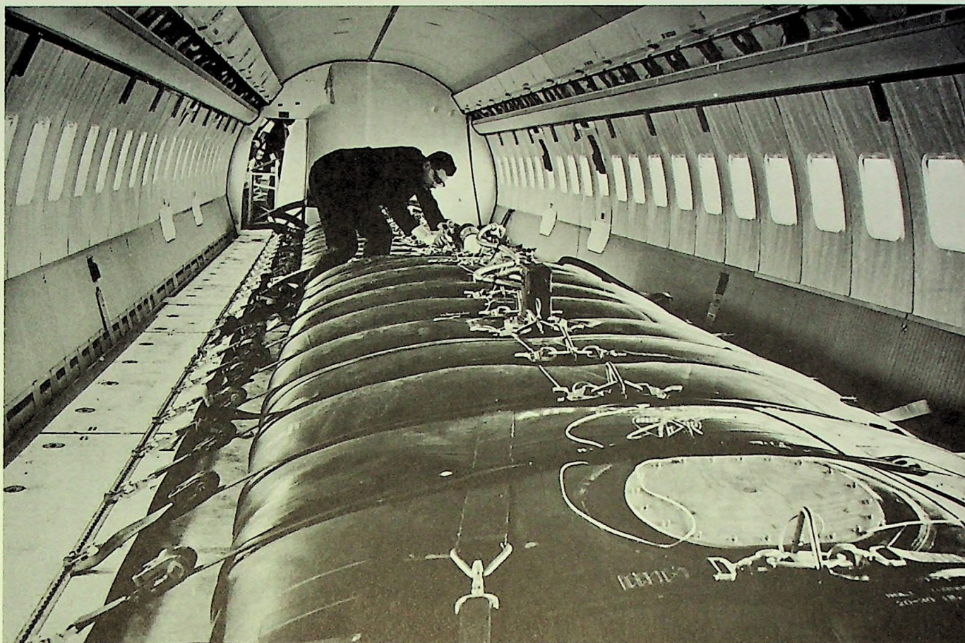
Special collapsible tanks for auxiliary fuel are installed inside the Boeing 707.
